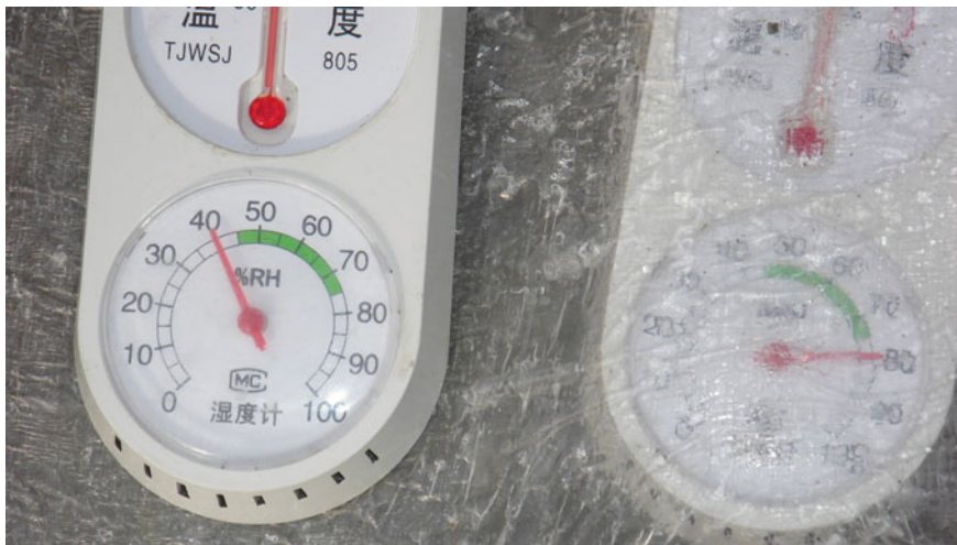
Fig. 3. Measurement of temperature and humidity of the inside and the outside of curing membrane. Notes The curing membrane was covered over concrete about 8 h later after the initial setting. The measuring time was from 0:10 to 17:00. The temperature during construction was 15–38 °C and the concrete ambient temperature was 18–44 °C
